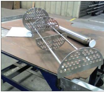
Figure 8. Condenser shell baffles.
