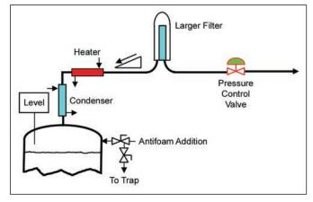
Figure 9. Exhaust heater.
