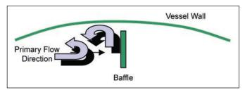
Figure 6. Formation of baffle vortexes.
