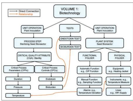
Figure 7. Schematic of a system, the seed bioreactor, and its equivalent process step.
