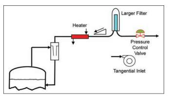
Figure 14. Vortex style foam separator.
