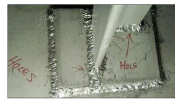
Figure 7. Bioreactor internal welds displaying defects.
