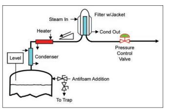
Figure 11. Exhaust filter with jacket
