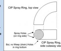
Figure 2. Schematic sketch of an internal CIP spray ring with no drain hole.
