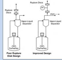
Figure 4. Poor rupture disc design and the
