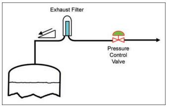
Figure 2. Simple exhaust path.
