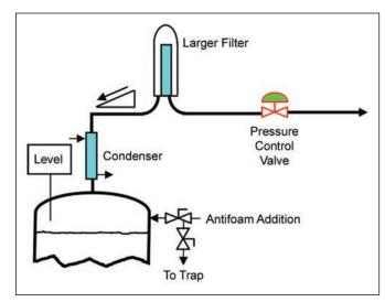
Figure 7. Condenser and larger filter area
