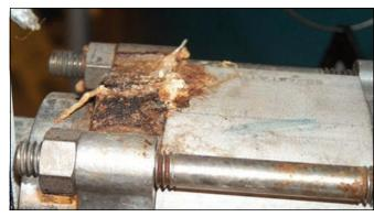
Figure 5. A leaking dextrose hand valve
