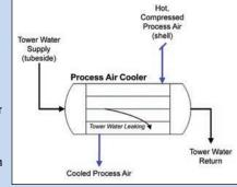
Figure 8. Compressed air cooler with a tower water leak.
