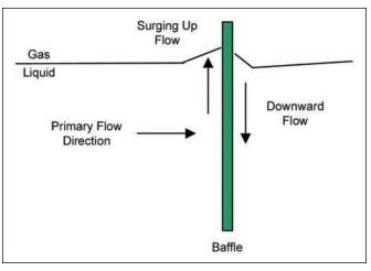
Figure 5. Liquid surge at baffles.
