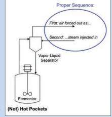
Figure 1. Displacing air with steam during fermentor SIP.
